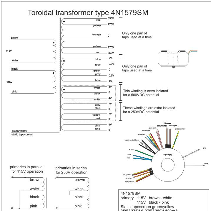
Diameter 125mm Height 41mm Weight 1.8kg
